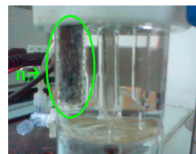
Figure 9. Control Potential Coulometry at -0.5 V vs NHE showing electrochemical \text{H}_2 generation from 0.5 \text{ N H}_2\text{SO}_4 using a cheap graphite electrode.
